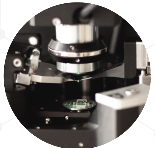
Probe and near-field antenna, with sample retracted
