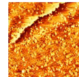
Figure 1: STM image (75 x 75 nm 2 ) of a FePc self-assembled layer on CoO/Ag(001).
